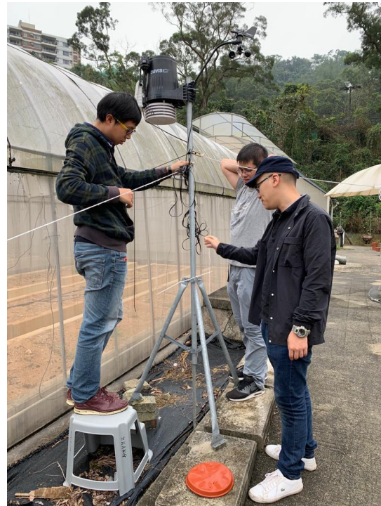
The team sets up a weather station in the ozone garden to monitor the micro-meteorology of the field site and the data is used for modelling the ozone impact on photosynthesis
